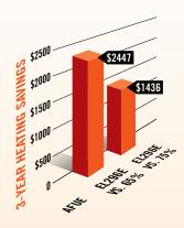
AFUE stands for "Annual Fuel Utilization Efficiency" and is a measure of a furnace's efficiency and performance. Like the miles-per-gallon rating on your car, the higher the AFUE rating, the lower your fuel costs. Most furnace ratings range from 80% to 95%.
